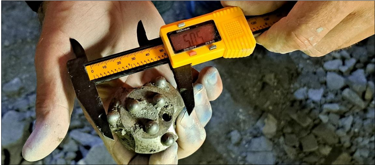
Figure 10 Rod anchor crown used for drilling exploratory wells
