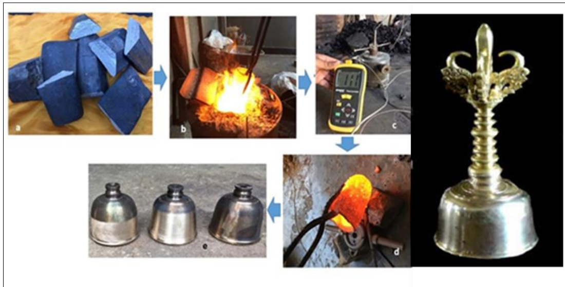
Figure 1 Mechanism of bell's production a. Bronze raw material. b. Process of smelting and preheating the molds c. Mold's temperature measurement. d. Pouring process. e. Bell product
