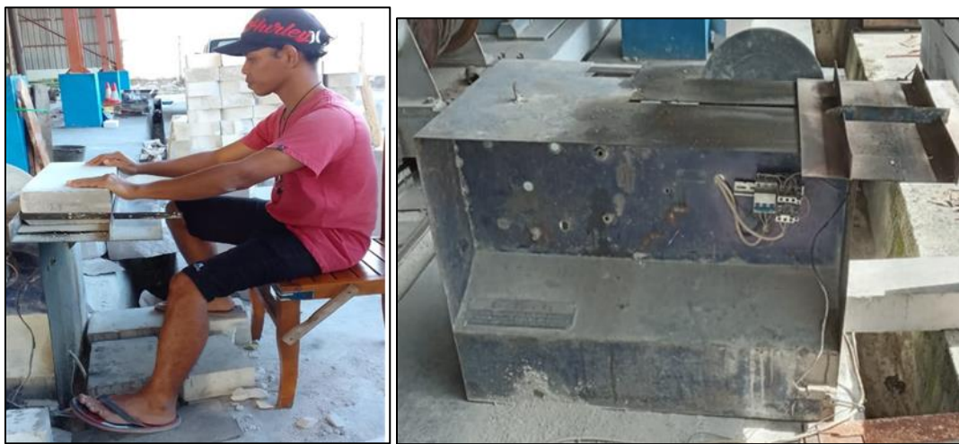
Figure 1 Worker working on a lightweight brick cutting machine before ergonomic intervention [14]
