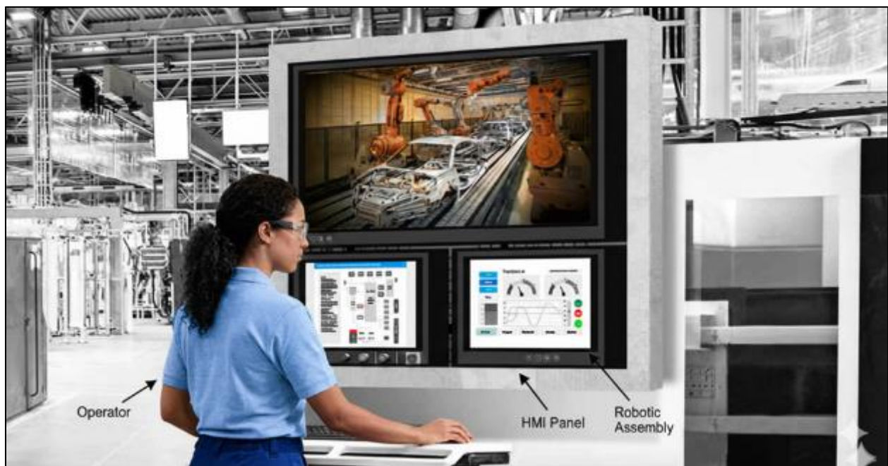
Figure 3 Touchscreen based human machine interface for workstation control
