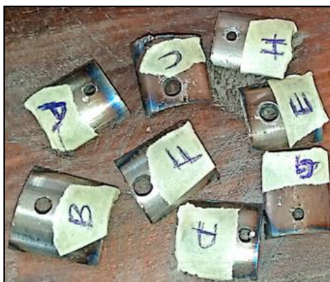
Figure 4 Some of the prepared samples used for the corrosion assessment tests
