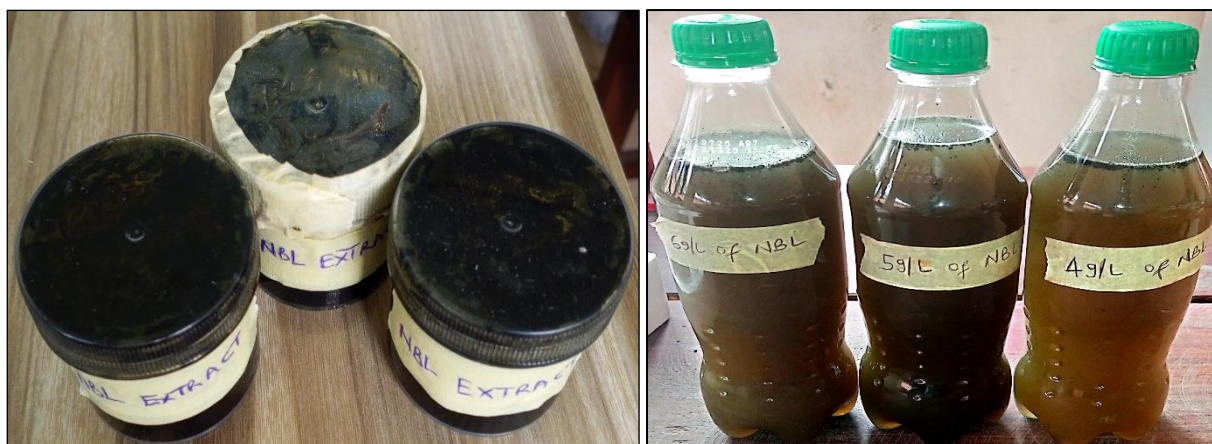
Figure 3 NBL inhibitor securely kept inside an airtight container (a) just as extracted from the Soxhlet machine (b) prepared to solutions of 4, 5, and 6g/l
