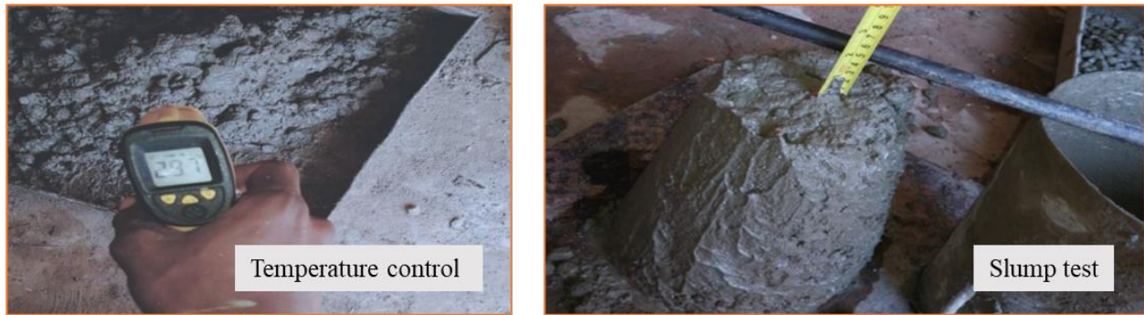
Figure 4 Temperature control and slump test configuration.
