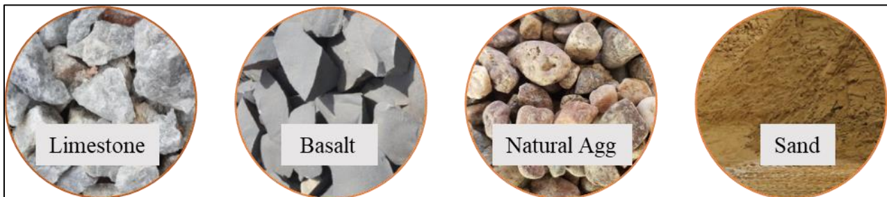
Figure 2 Materials used to produce M25 grade concrete.
