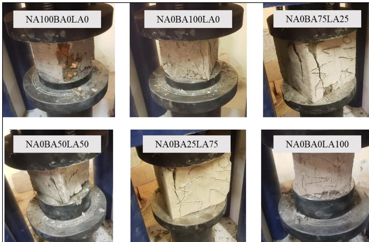
Figure 7 Failure modes of cube specimens
