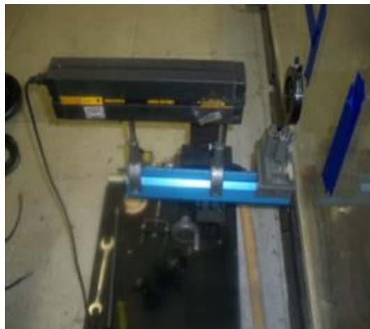
Figure 15 20 mw Coherent Laser
