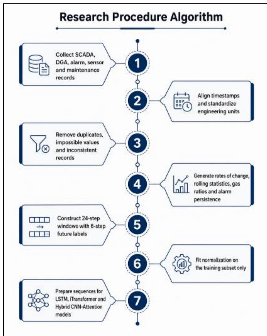
Figure 2 Research procedure algorithm for data preparation, model training, validation and decision support
