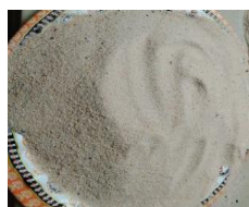
Figure 1I sand (1.00mm particle size)
