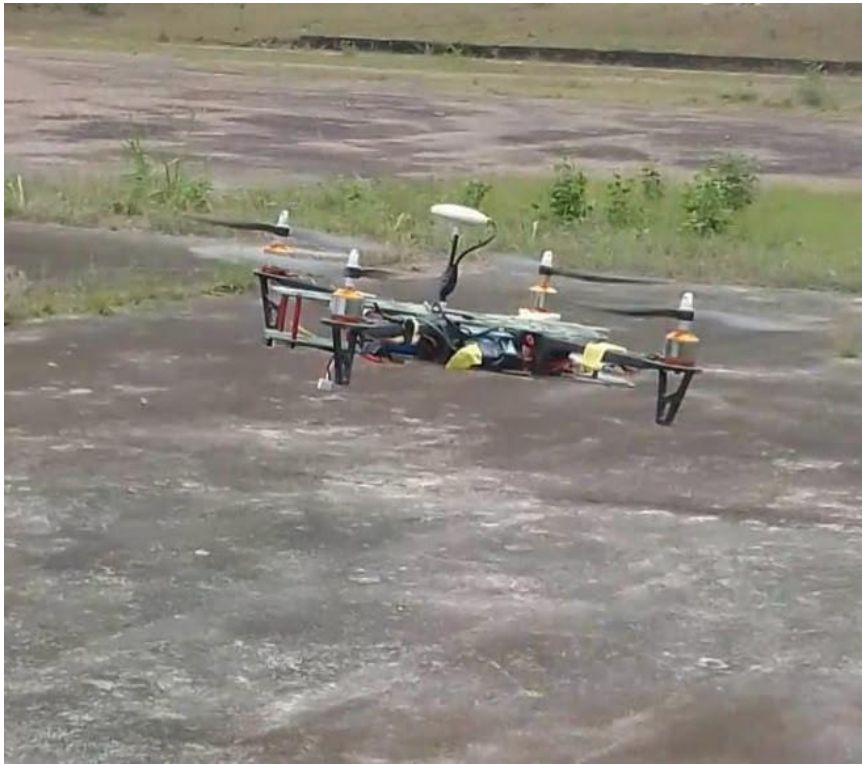
Figure 4 Photograph of the assembled quadcopter platform during outdoor hover/flight testing, corresponding to the physical parameters of Table 2.
