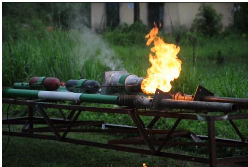
Figure 7 The designed liquid rocket engine static test
