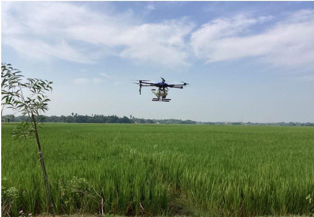
Figure 1 The quadcopter platform conducting an autonomous multispectral survey over a rice paddy test field.
