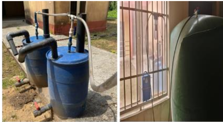
Figure 2: The complete fabricated biogas digester.
