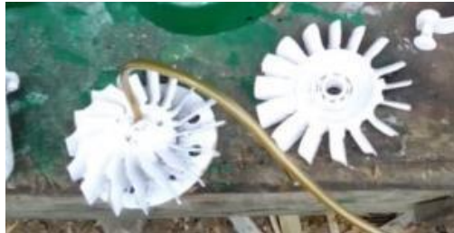
Figure 9: Machined compressor and turbine rotor blades prior to shaft assembly.
