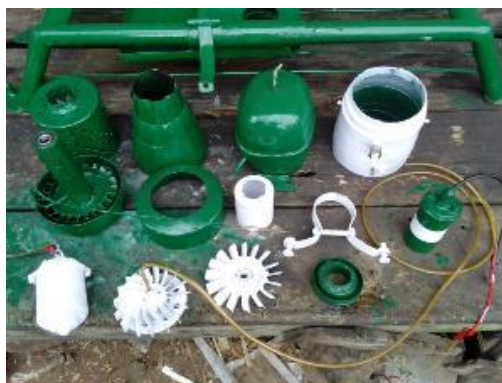
Figure 11: Overview of the fabricated auxiliary jet engine components prior to final assembly, including the fuel tank, exhaust cone, combustion-chamber housing, compressor/turbine rotors, mounting clamp, and igniter module.
