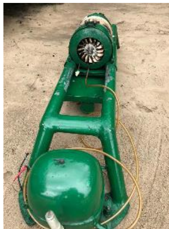
Figure 14: Fully assembled auxiliary jet engine mounted on its support frame with fuel tank and ignition wiring installed, prior to test firing.
