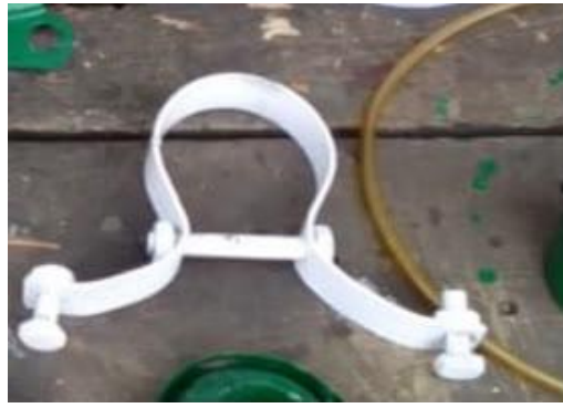
Figure 12: Mounting clamp fabricated for securing the engine housing to the airframe support structure.
