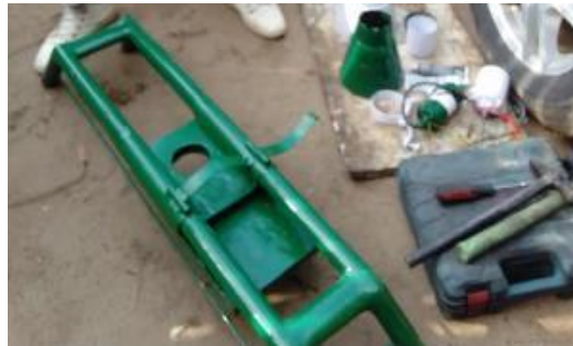
Figure 13: Fabricated engine support frame/mount rail, shown alongside additional components and assembly tools.
