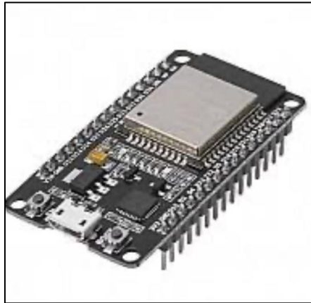
Figure 3: ESP32 development board (ESP32-WROOM-32 module), used as the representative MCU part for Table I.
