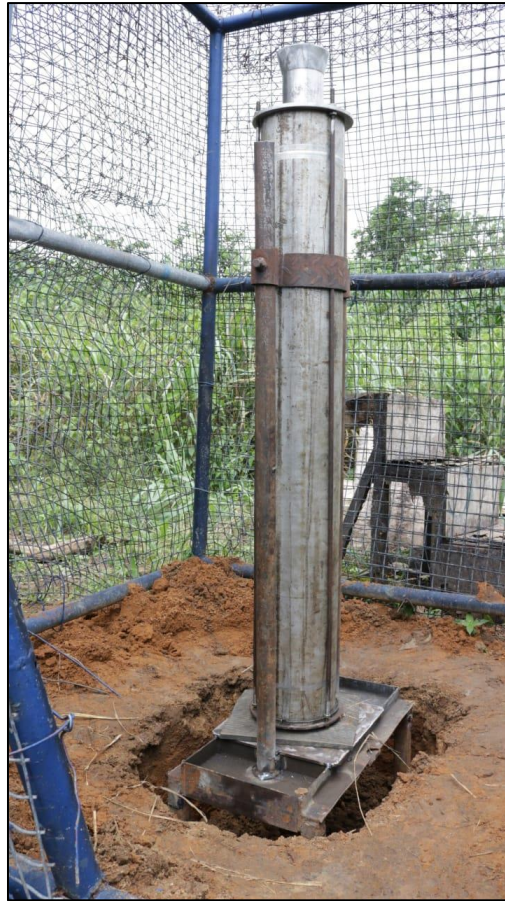
Figure 2: The same small-scale test-stand motor secured vertically within a protective wire-mesh safety cage prior to ignition, illustrating the ground-restraint and stand-off enclosure used for personnel protection during the small-motor/educational test described above.
