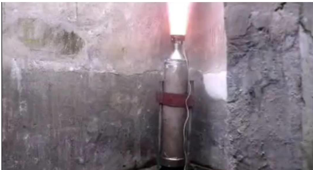
Figure 1: A restrained, guy-wired small-scale static fire test stand during ignition, illustrating the exhaust plume, ground-restraint hardware, and stand-off distance characteristic of the small-motor/educational methodology described above. (Illustrative photograph; not associated with a certification-grade facility.)
