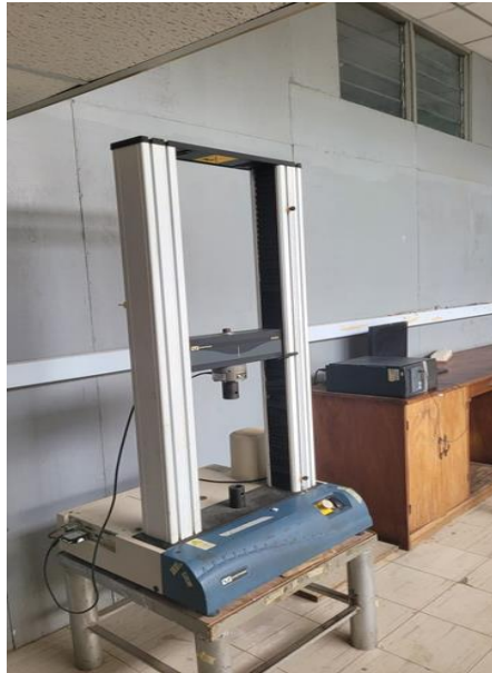
Figure 2: Universal Testing Machine used for Flexural Testing
