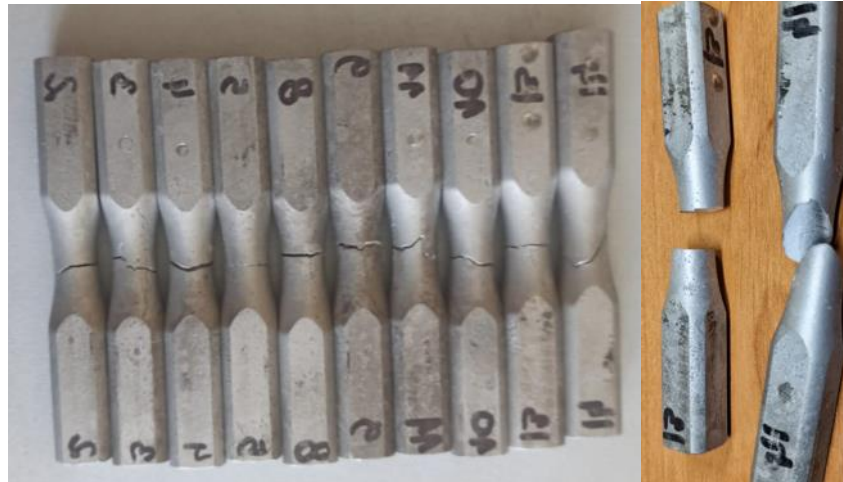
Figure 3: Fractured specimens (Figure 4) Fracture surfaces (close-up view)
