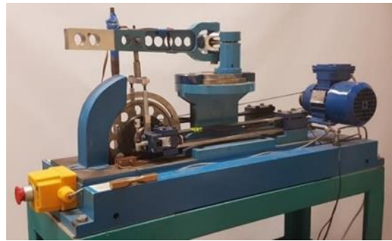
Figure 2: The Actelelik MZGS-100 fatigue testing machine equipped for bending and torsion loading was used in this study.
